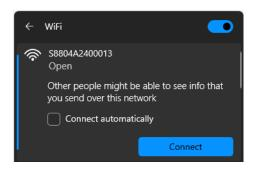
Once connected with a smartphone or PC, using any internet browser the WebUI is found at the IP address: 192.168.10.1
