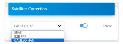
Once enabled, the device will start using the corrections received from the satellites to improve the quality of the position.
