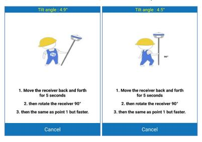
If the screen does not disappear, try changing the position to get lower RMS values and then repeat the two steps.
