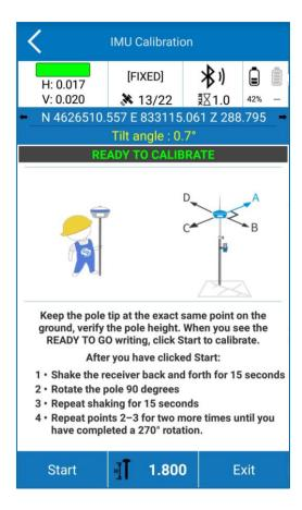
The calibration consists of the same movement repeated along the four orthogonal directions while keeping the pole tip on the same point on the ground:
