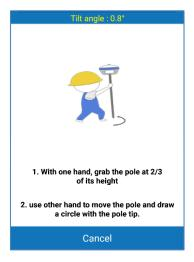
The second screen shows how to aid the sensor to adjust the calibration parameters based on the local GNSS position and accuracy.
