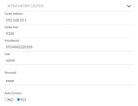
The caster address and port cannot be changed. Mountpoint, User and Password can be changed. The default values are:
